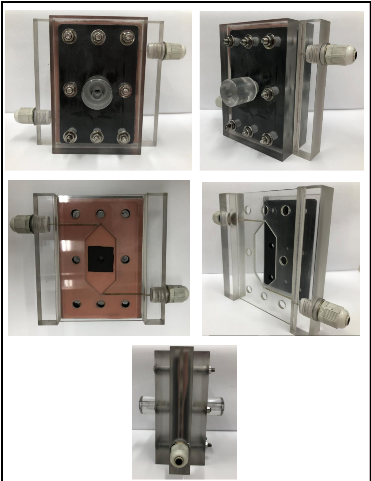
Figure 7.1. Detailed photos of the flow-by cell (FBC).
