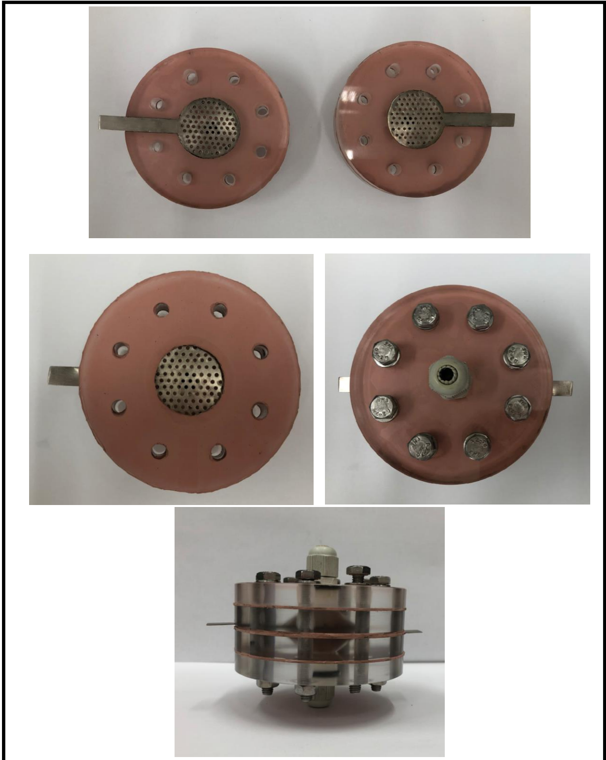
Figure 7.2. Detailed photos of the flow-through cell (FTC).
