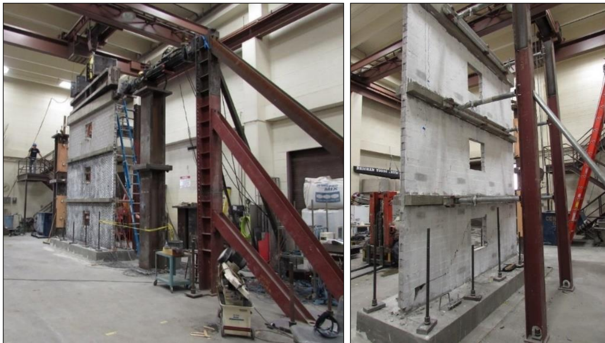
(a) The actuator and in-plane supports
