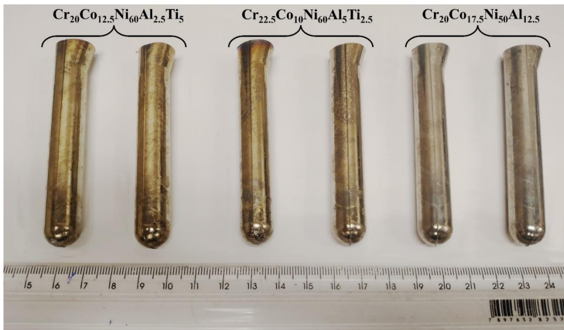
Figure 5.16: Ingots of \text{Cr}_{20}\text{Co}_{12.5}\text{Ni}_{60}\text{Al}_{2.5}\text{Ti}_5 , \text{Cr}_{22.5}\text{Co}_{10}\text{Ni}_{60}\text{Al}_5\text{Ti}_{2.5} , and \text{Cr}_{20}\text{Co}_{17.5}\text{Ni}_{50}\text{Al}_{12.5} alloys produced in an Arc-Melter furnace.
