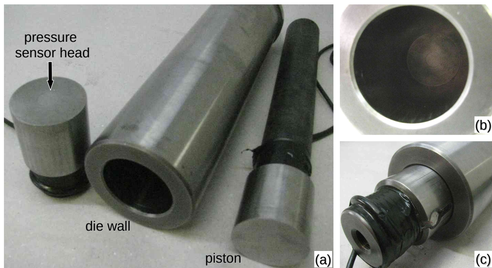
Figure 3.4 Photographies of the (a) metal rigid die and (b,c) details of pistons-die walls assembly [56]
