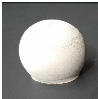
Figure 4.30 Ceramic femoral head produced via RMP.
