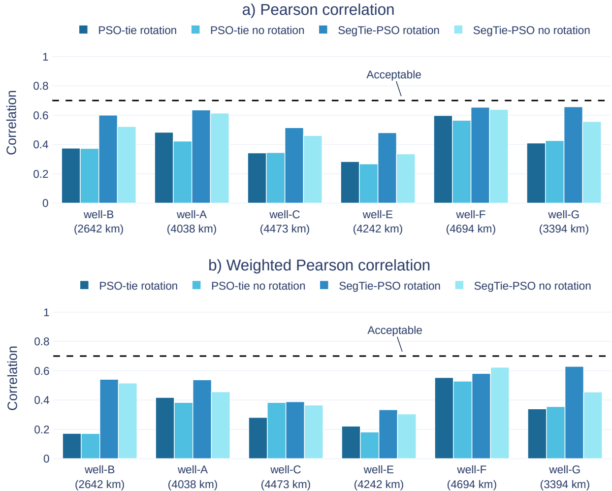
Figure 34 – Performance of the PSO-tie and SegTie-PSO. a) Presents the correlation obtained using the Pearson correlation as a cost function, while (b) uses weighted Pearson correlation.
