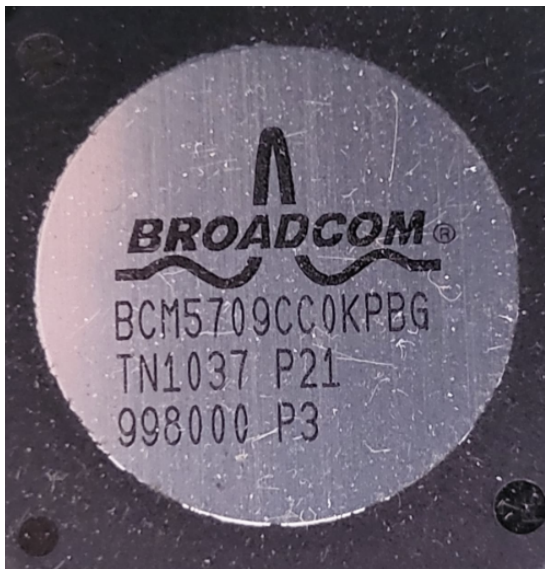
(a) Chip principal da Placa de rede Broadcom BCM5709CC0KPBG.
