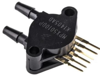
(b) Piezoresistive transducer MPX5010dp pressure gauge.
