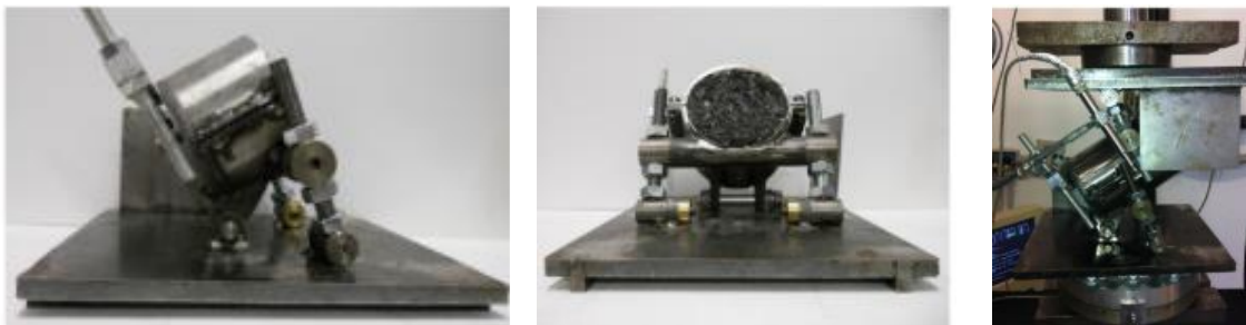
Figure 2.27 – Sapienza Inclined Shear Test Machine. Source: D’Andrea and Tozzo (2016).
