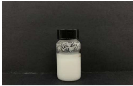
Figure15 Cellulose acetate solution for electrospinning
