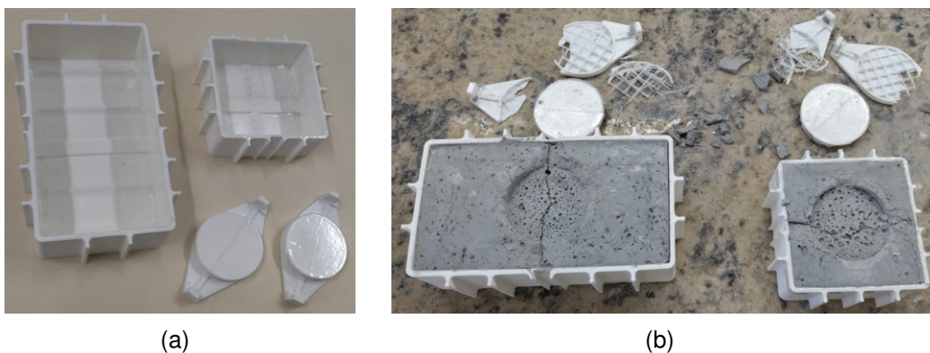
Figure 3.9: (a) First empty molds made of PLA for producing loading parts from refractory mortar and (b) during unmolding with cracked refractory parts.
