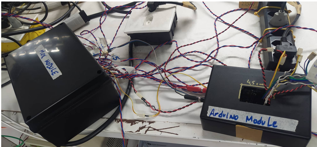
Figure A.1: Photo of the final project modules operating at our lab. The circuit functions through two distinct modules: Arduino and Mux. The Arduino Module not only accommodates the Arduino component but also includes the supply voltage regulator. In contrast, the Mux Module houses the multiplexer and the MAX6675 temperature sensor. These modules are interlinked through Molex connectors, facilitating troubleshooting efforts for each module individually.
