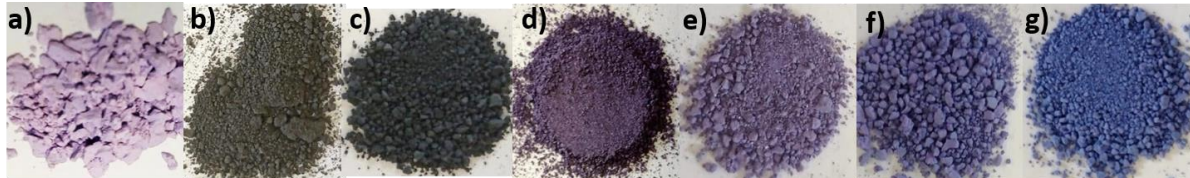
Figure 12: Powders produced by spray drying of the solution S100M a) as-sprayed, b) after drying at 600 °C and after heat treatment at c) 800 °C, d) 850 °C, e) 900 °C, f) 950 °C and g) 1000 °C.
