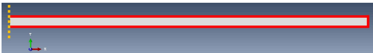
Figure 7 – Boundary conditions on axisymmetric model of the disc's half cross-section.
