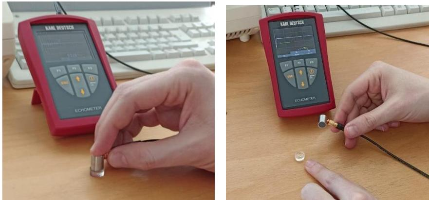
**Figura 16:** Equipamento ultrasonic path length (*ECHOMETER Karl Deutch, Hürth, Germany*).
