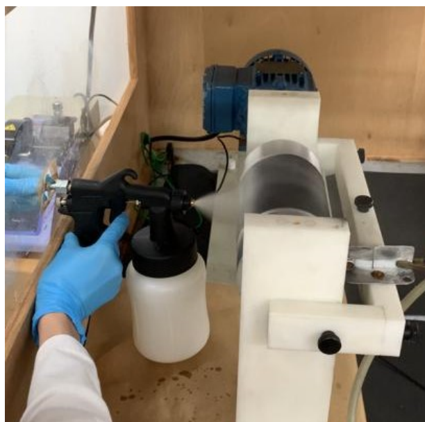
Figure 6.2 – Experimental apparatus for coating membranes with \text{CuSO}_4 and CuNP.
