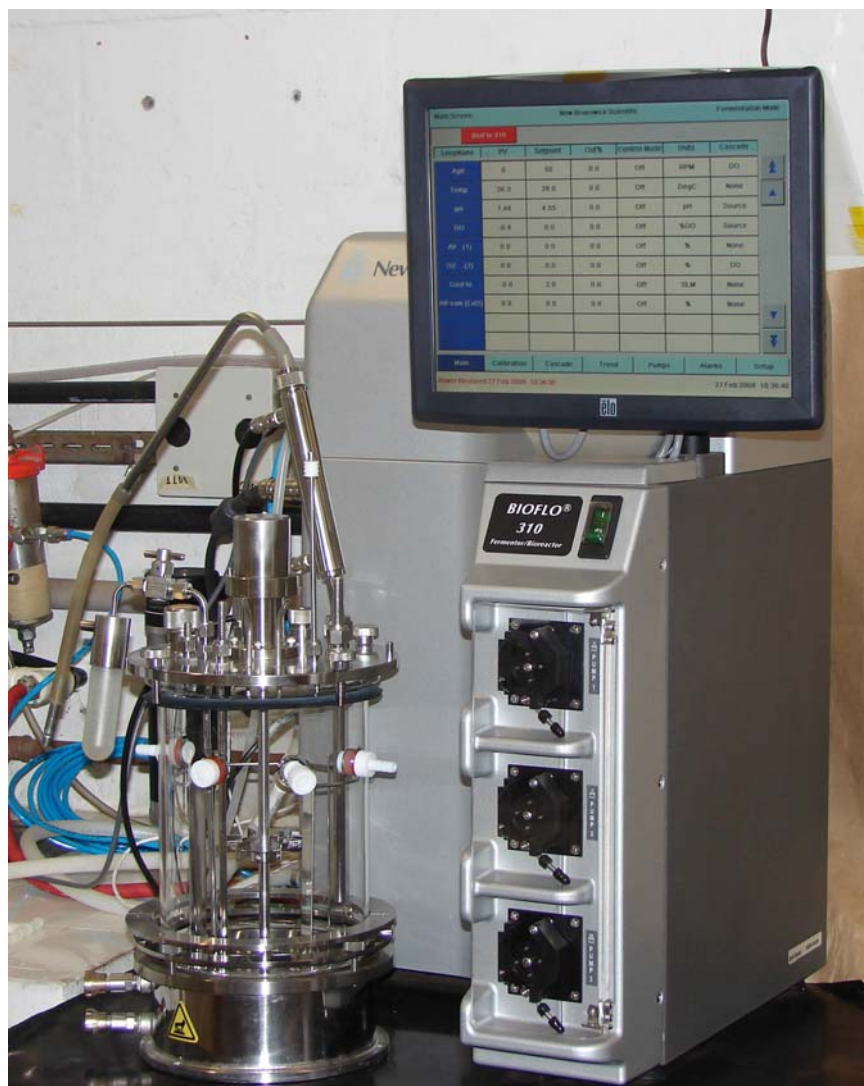
Figura 3.1: Biorreator Bioflo 310 com dorna de 5L, New Brunswick Scientific
