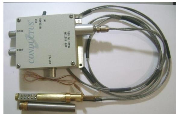
Figura 5.35: O iFL-301 Flux-Locked Loop e o MFP.
