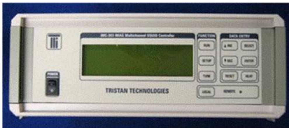
Figura 5.38: Panel frontal do controlador do S.Q.U.I.D. iMC-303 multicanal da Tristan Technologies.
