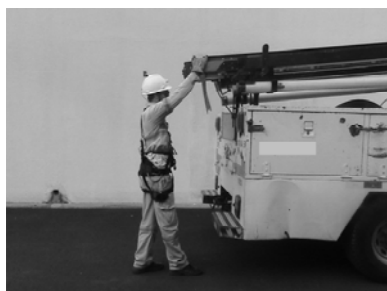
Fig. 1. Overhead loading and unloading a truck ladder by a line worker (ladder support is at 1.70 meters above the ground).
