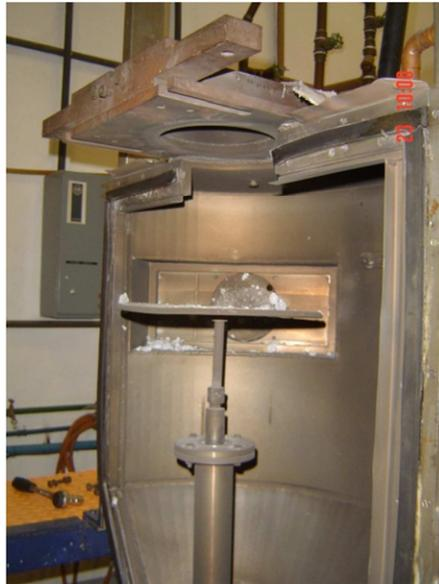
Figura 13 – Câmara de Sprayforming.
