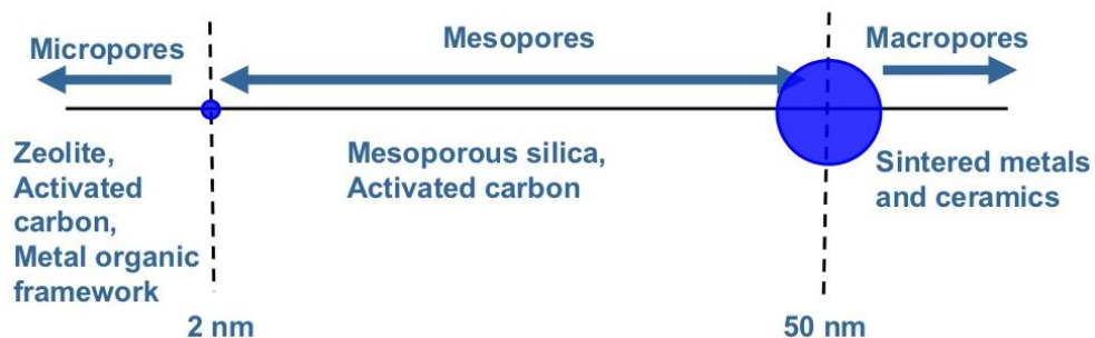
Figure 2.3 Classification of porous materials by pore size according IUPAC standard [25].
