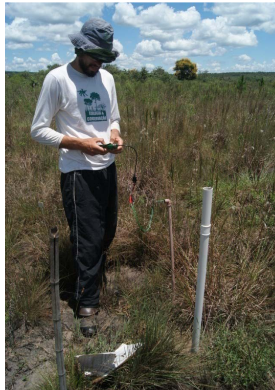
Figure 4 – Images of sampling methods in the Itirapina Ecological Station. up – experimental 10 x 10 plot with 1 x 1 subplots. bottom left – Drilling to the water table. bottom right – Measurement of water potential in one plot, also showing the PVC pipe into which the tape was introduced to measure the depth to the water table.
