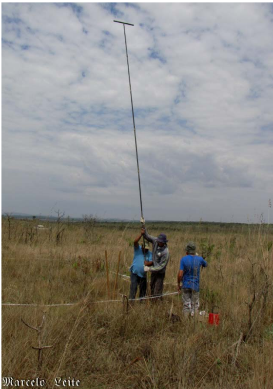
Figure 4 – Images of sampling methods in the Itirapina Ecological Station. up – experimental 10 x 10 plot with 1 x 1 subplots. bottom left – Drilling to the water table. bottom right – Measurement of water potential in one plot, also showing the PVC pipe into which the tape was introduced to measure the depth to the water table.
