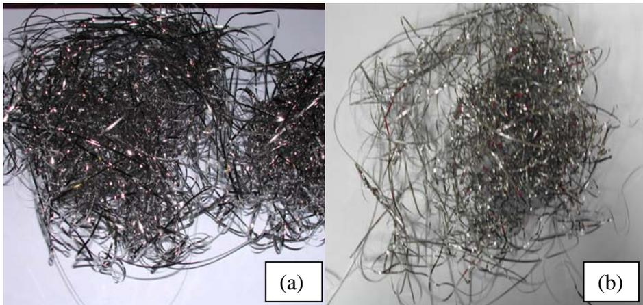
Figura 4.2 Aspecto visual externo das fitas produzidas por melt-spinning (a)  $(\text{TiZr})_{80}\text{Co}_{12}\text{Fe}_8$  (b)  $\text{Ti}_{34}\text{Ni}_8\text{Cu}_{36}\text{Zr}_{22}$ .
