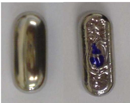
Figura 4.1 Lingotes das ligas  $(\text{TiZr})_{80}\text{Co}_{12}\text{Fe}_8$  e  $\text{Ti}_{34}\text{Cu}_{36}\text{Ni}_8\text{Zr}_{22}$ .
