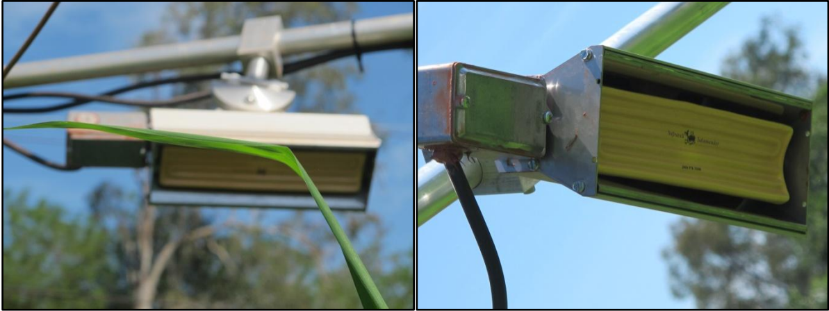
Fig. FACE 19. Heaters model FTE-750-240 Salamander ceramic infrared heating elements, mounted on Salamander ALEX-F reflectors (Mor Electric, MI, USA) suspended at 0.8 m above the canopy.
