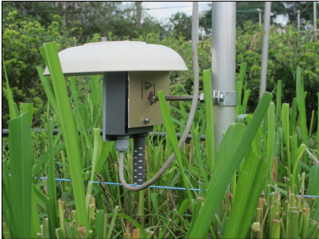
Fig. FACE 14. CARBOCAP infrared gas analyzer (IRGA) Model GMP 343 (Vaisala, Finland).
