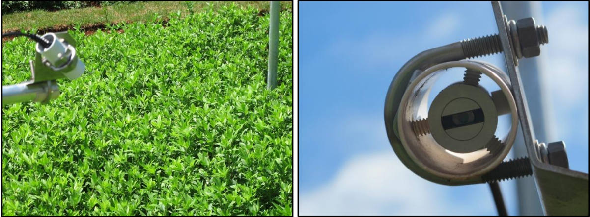
Fig. FACE 20. Infrared thermometer model SI-1H1-L20 (Apogee Instruments, USA).
