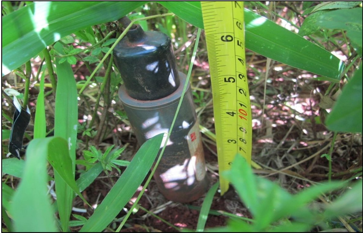
Fig. FACE 22. Theta Probe soil moisture (ML2x) and temperature (ST2) sensors.
