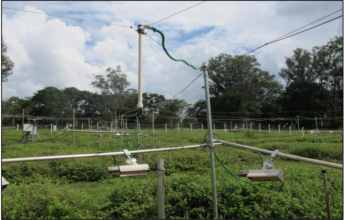
Fig. FACE 24. Water sprinklers suspended at the center of the plot.
