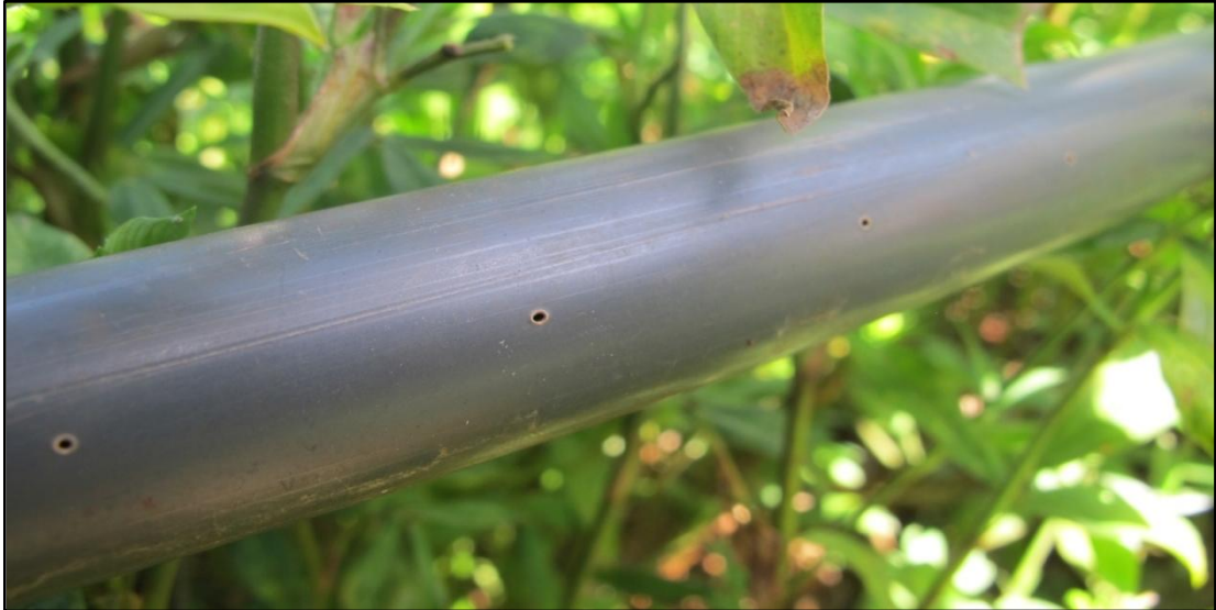
Fig. FACE 17. CO 2 fumigation micro holes in outer ring side surrounding each plot.
