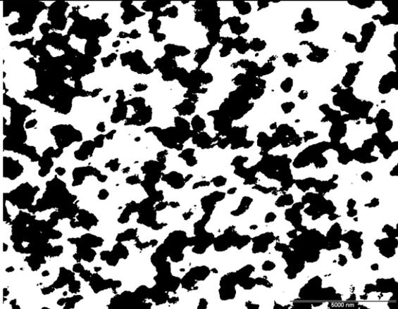
A binary (black and white) version of the micrograph, where the dark particles are represented as solid black shapes on a white background. A scale bar in the bottom right corner indicates 5000 nm.   |
