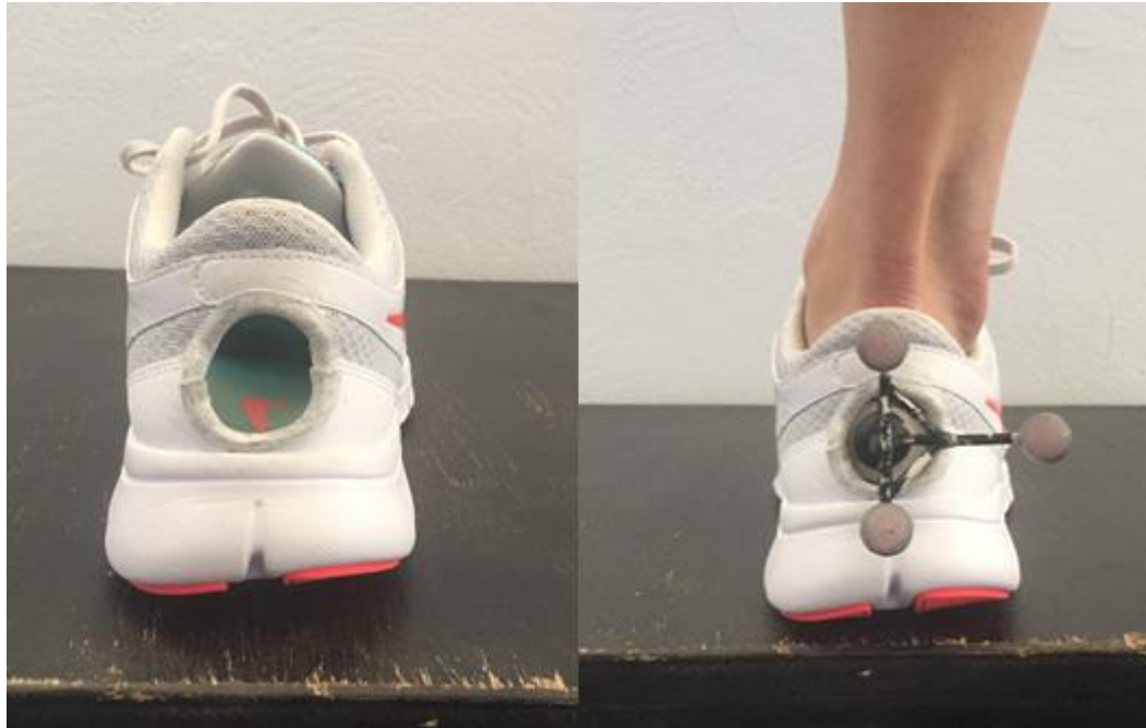
Fig. 1. Custom running shoe with opening in the posterior region to place the cluster directly on the calcaneus.
