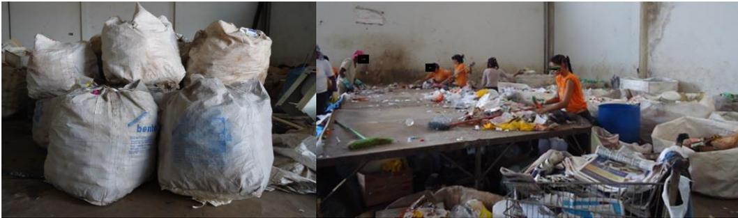
**Figure 1.** **A** Bags with recyclable materials to be sorted; **B** Workers sorting the materials in the fixed work surface.
