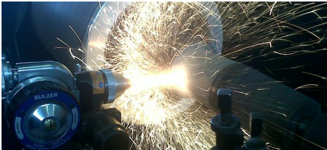
Figura 2.11: Processo de Flame Spray. [38]
