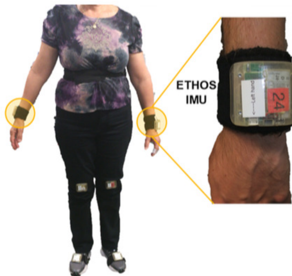
Figure 2.4: A subject wearing the system used to design the CuPid dataset, with focus on the IMUs attached on the wrists. Extracted from (MAZILU; BLANKE; TRÖSTER, 2015).
