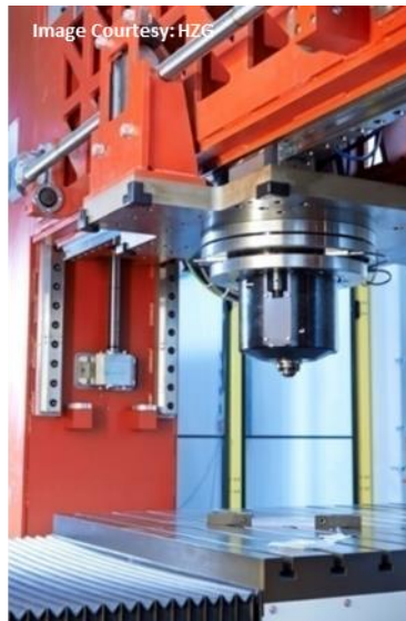
Figure 2.9 Friction Riveting equipment (commercially available high-speed friction- welding spindle on automated structure with tri-axial force sensors and an integrated position sensor) available at Helmholtz Centre Geesthacht, Germany.
