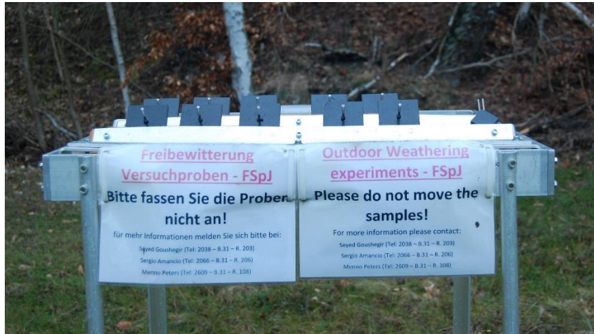
Figure 3.9 Natural weatherability testing jig for the friction-riveted AA6056-T6/PA6-30GF joints.
