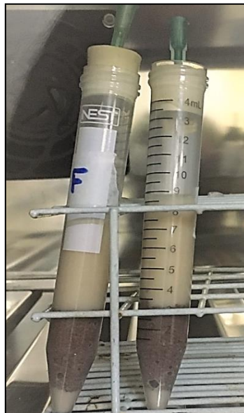
Figure SM2. Mini-reactors containing cell suspension and commercial xylose isomerase IGI-HF.
