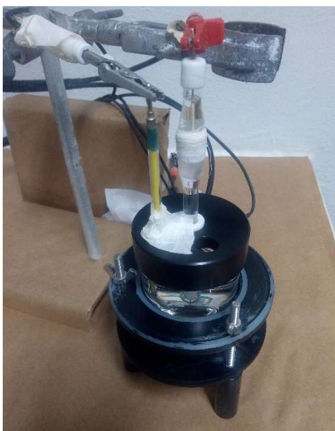
Figure 3.9 – Electrochemical cell setup for PP and EIS tests. Source: author.
