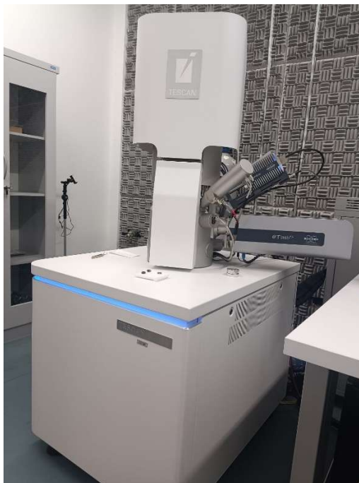
Figure 3.5 – TESCAN MIRA microscope coupled with a Bruker EDS detector. Source: the author.
