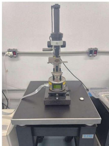
Figure 3.6 – AFM Bruker Nanoscope V Multimode ScanAsyst. Source: author.
