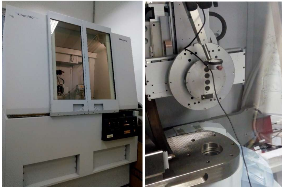
Figure 3.4 – Diffractometer PANalytical X'Pert PRO, MRD-XL. Source:author.
