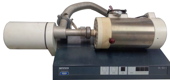
Figure 3.15: NETZSCH - DIL 402 C push rod dilatometer used for measurement of the material samples CTE.
