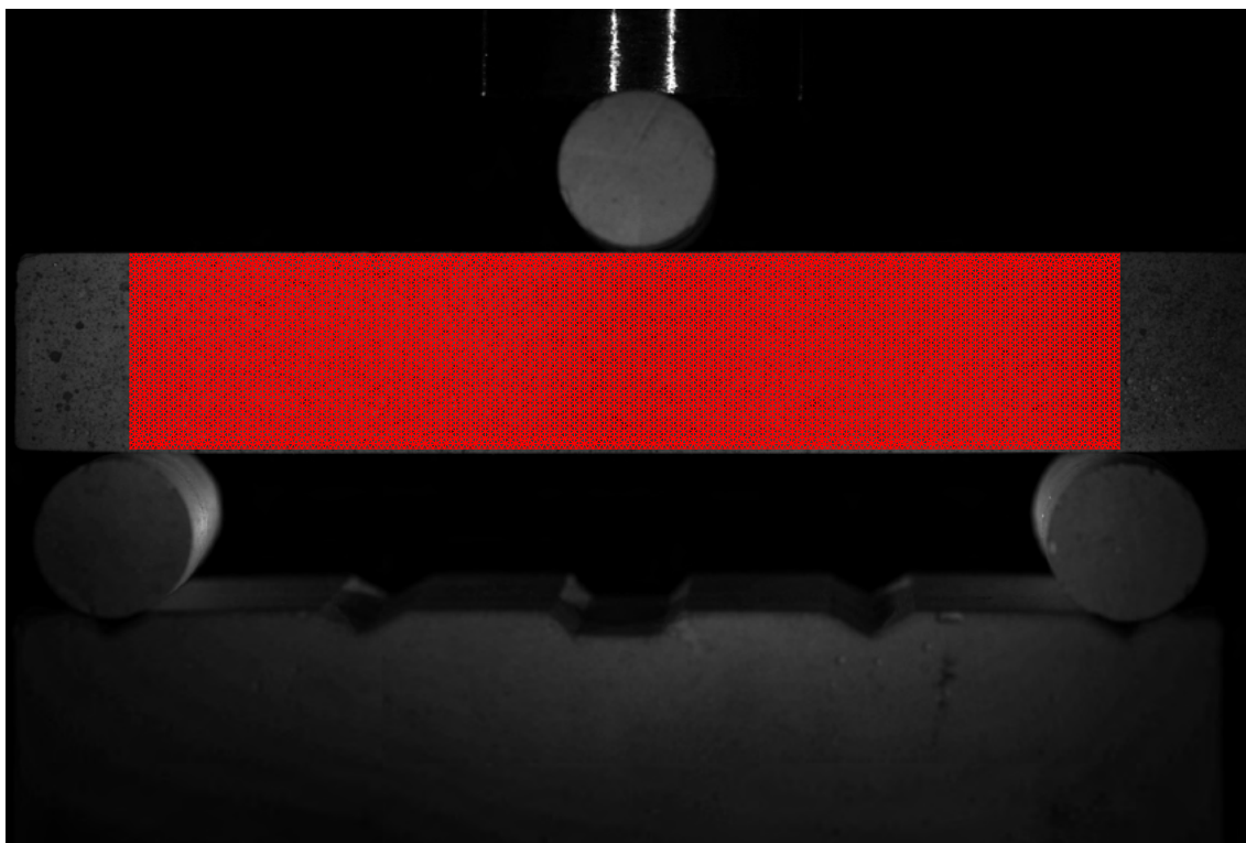
Figure 4.10: Mesh used for the correlation of one of the EA-B1 specimen's faces.
