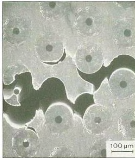
Figure 1.3: Cracks in a titanium metal matrix reinforced with silicon carbide fibers. (credits: J G Robinson and British Petroleum) [35].
