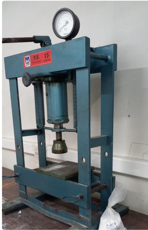
Figure 3.11: Pressing machine used to produce specimens of atomized alumina and zirconia.
