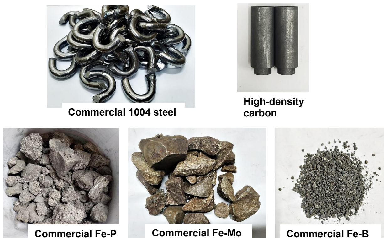
Figure 3.2- Commercial materials used to produce the Fe-Mo-P-C-B alloys.
