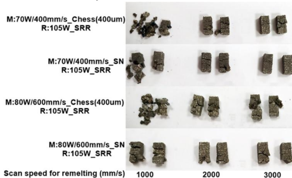
Figure 4.29- LPBF samples produced using different combinations of parameters for melting and remelting, as specified in the image. The influence of different (1000, 2000, and 3000 mm/s) scan speeds for the remelting is shown.
