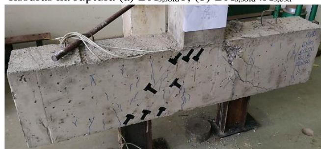
(b) BA_{s,sold}4A_{s,estr} : face frontal - fissuras na ruptura
