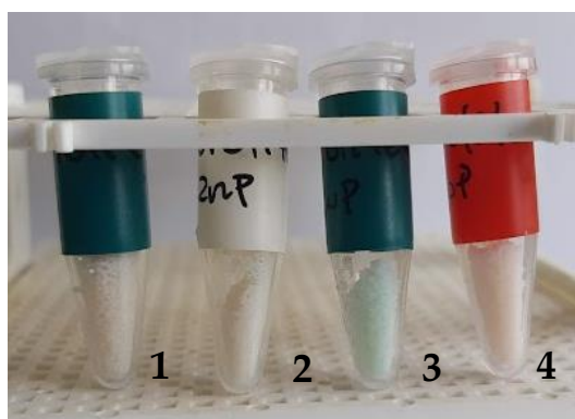
Figure 5.3. Purolite C18 TLL (1) unmodified modified with (2) \text{ZnCl}_2 /sodium phosphate, (3) \text{CuCl}_2 /sodium phosphate and (4) \text{CoCl}_2 /sodium phosphate. Other specifications are described in Methods.
