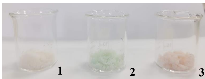
Figure A3.9. Purolite-TLL (20 mg/g) modified with (1) \text{ZnCl}_2 /sodium phosphate, (2) \text{CuCl}_2 /sodium phosphate and (3) \text{CoCl}_2 /sodium phosphate. Other specifications are described in Methods.
