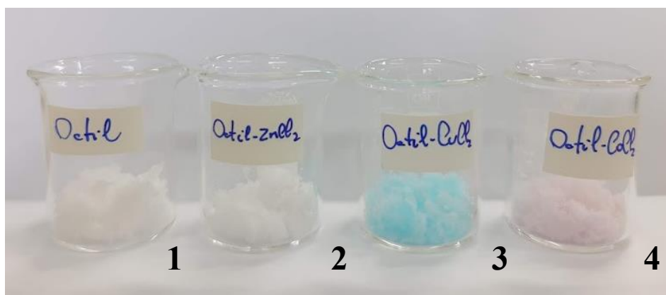
Figure A3.4. TLL (1 mg/g) immobilized on (1) octyl agarose and (2-4) octyl agarose modified with: (2) ZnCl 2 /sodium phosphate, (3) CuCl 2 /sodium phosphate and (4) CoCl 2 /sodium
