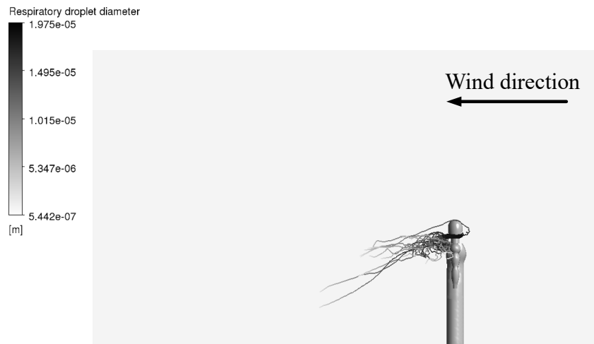
Figure 43- The flow profile of smaller respiratory droplets of 50 \mu\text{m} in diameter using no-slip stress boundary condition and (a) 0.5 m/s (b) 1 m/s and (c) 3 m/s velocities
