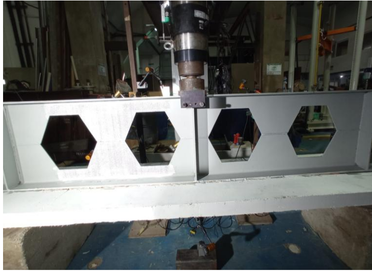
(a) CCB-P specimen (view from side B and DIC's view)
