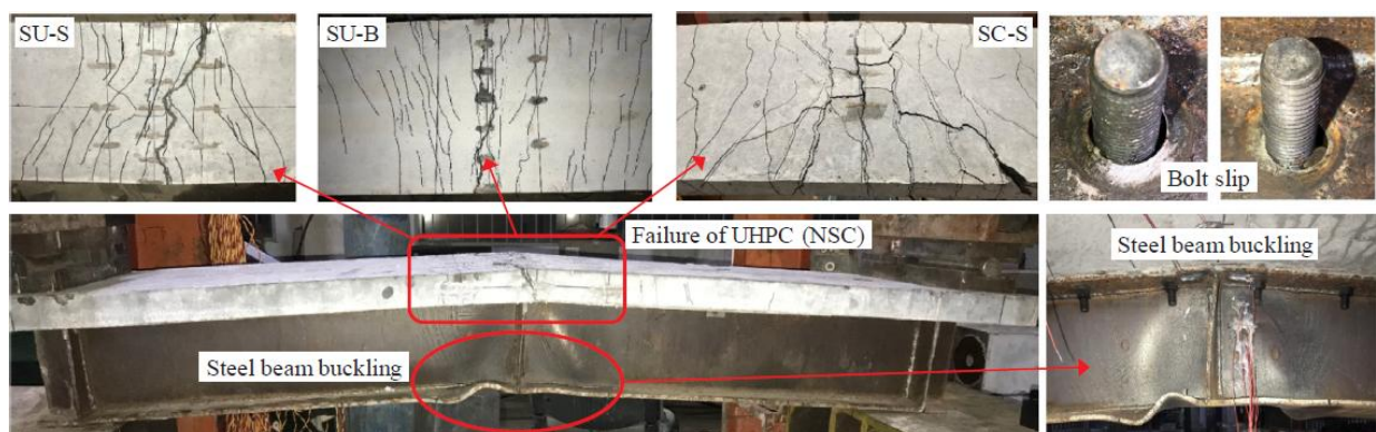
Figure 2.21: Three-point bending tests by Zhang et al. (2020).
