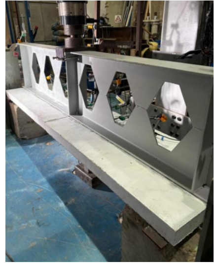
(b) CCB-P specimen (DIC's side)
