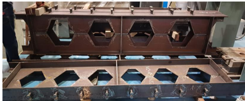
(d) Manufactured steel castellated I-beams with headed studs welded in the top flanges
