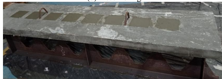
(c) Cast shear pocket
