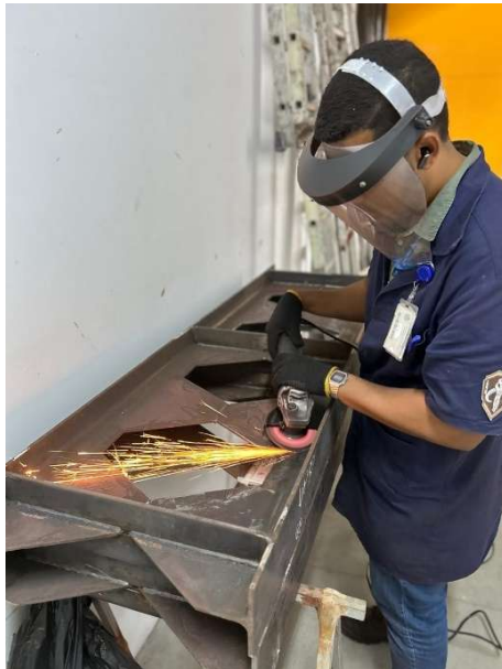
Figure 13 - Cleaning beam process.
