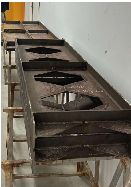
c) Manufactured steel castellated I-beams.
