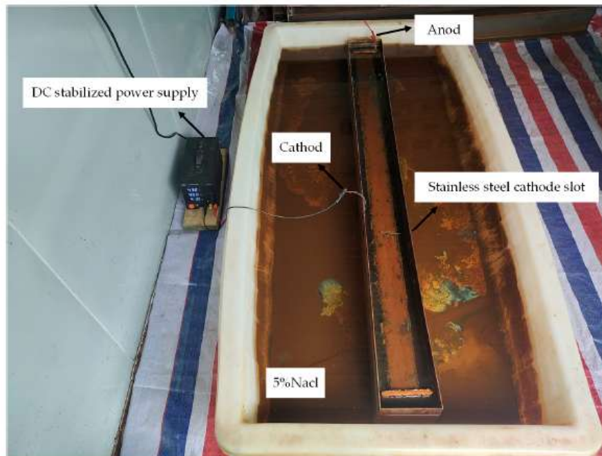
Figure 06. Electrochemical corrosion test.
