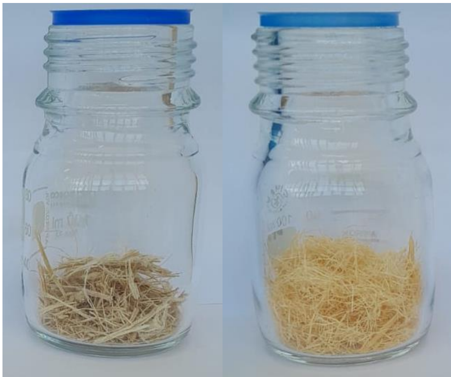
Figure 6. 2 - Physical appearance of sugarcane bagasse (1g): (left) untreated and (right) pretreated with hydrogen peroxide and acetic acid for 4 h at 60 °C and 100 rpm.
