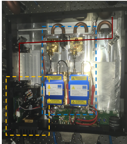
Figure 16 – Inside the Mephisto laser showing the Master Oscillator (MO) inside the yellow box, the Power Amplifier (PA) inside the blue box and the laser light path on dark red.
