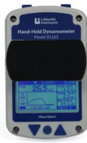
Figura 2. Dinamômetro manual (Lafayette Model-01165, Lafayette Instrument Inc, USA).
