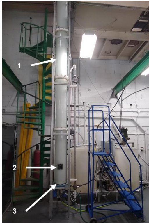
Figure 2.2. Reactor or gas/liquid contactor of 180 L used in the experiments. (1) the reactor, (2) a flat black plate used as a background for image acquisition, and (3) the sparger of FBG system brought from Brazil.
