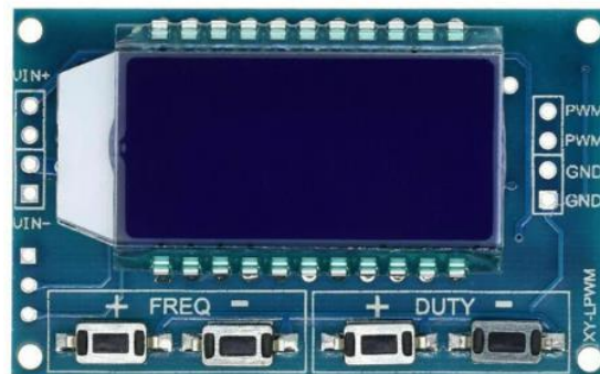
Figure 2.4. PWM module to control the solenoid valve.
