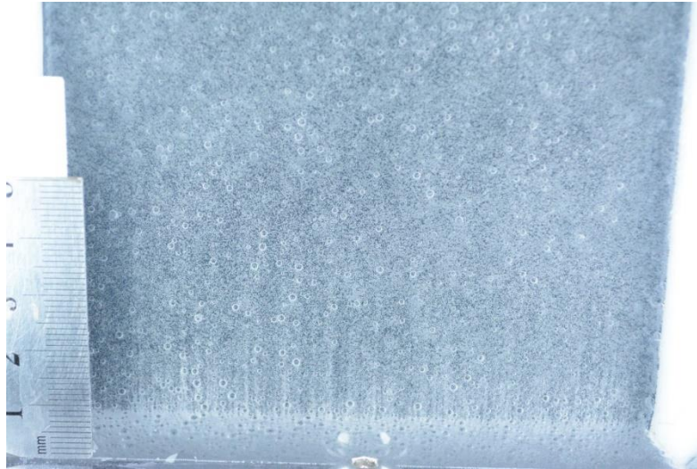
Figure 4.10. Microbubbles generated by the SSD sparger at 3.0 \text{ L min}^{-1} .
