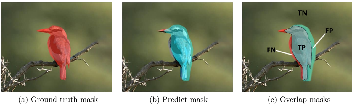
Figure 9 – Visual representation of the confusion matrix components in segmentation. Adapted from (KUKIL, 2022).
