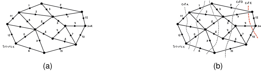
Fig. 1. Representation of a large-scale flow network, showing source(s), sink(t), and various possible slices. (a) source node and sink node. (b) graph cuts
