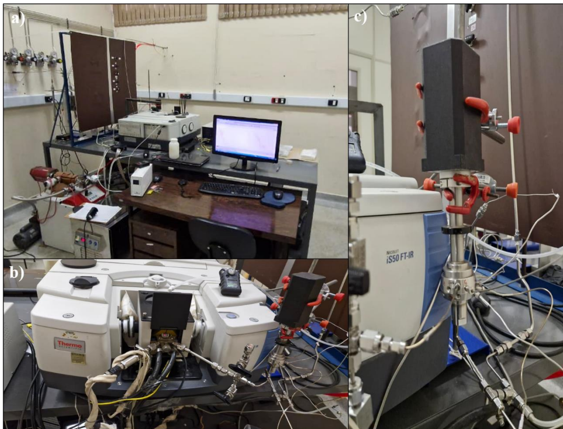
Figure 2. System designed for ME-PSD-DRIFTS experiments
