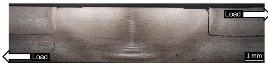
Figure 3.27 - Sheet thickness fatigue crack propagation by the base material and between SZ/TMAZ interface [18].
