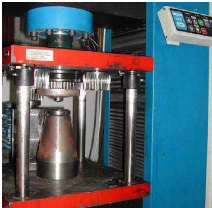
Figure 15: Universal Testing Machine EMIC and HPT accessory.
