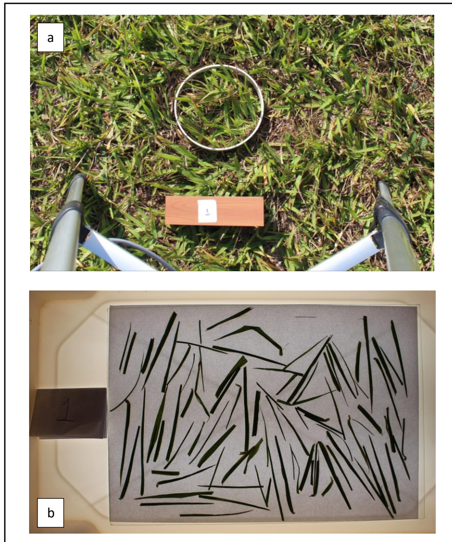
Figure 16: (a) the view angle (80°) of the ASD FieldSpec measurements above one of the circular sites; (b) Example of photographs taken in the experiment for leaf area estimation by ImageJ software.
