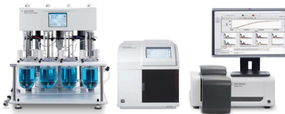
FIGURE 11. Agilent scanning UV dissolution system with an online Cary 60 –UV-Vis Spectrophotometer.
