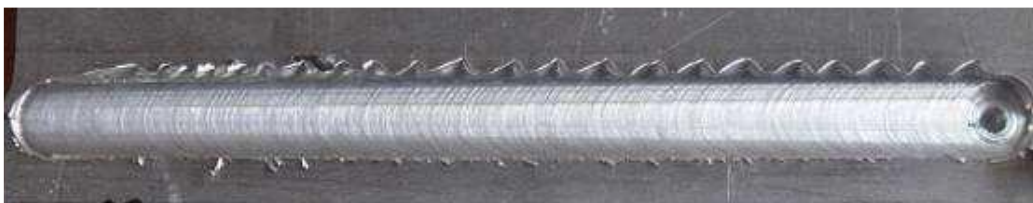
Figure 3.17 - Top view of AA2XXX welded by FSW showing excessive flash formation on the side of the weld. Image courtesy of Helmholtz-Zentrum Geesthacht.
