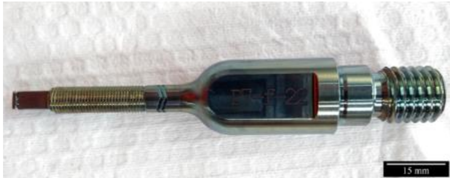
Figure 4.2 - Image of probe used during welding. Image courtesy of Helmholtz-Zentrum Geesthacht.
