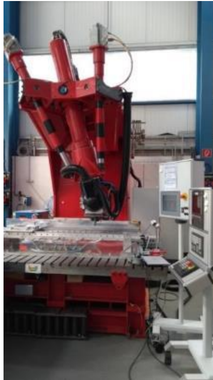
Figure 4.4 - PKM T805 machine equipped with a custom design BT-FSW spindle.
